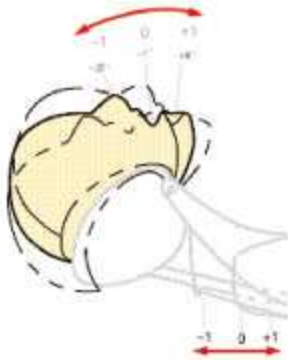
Fig. 4 An ergonomic headrest provides the best access to the mouth, finger stability, and views of the mouth with a few simple adjustments in the "Y" plane.
